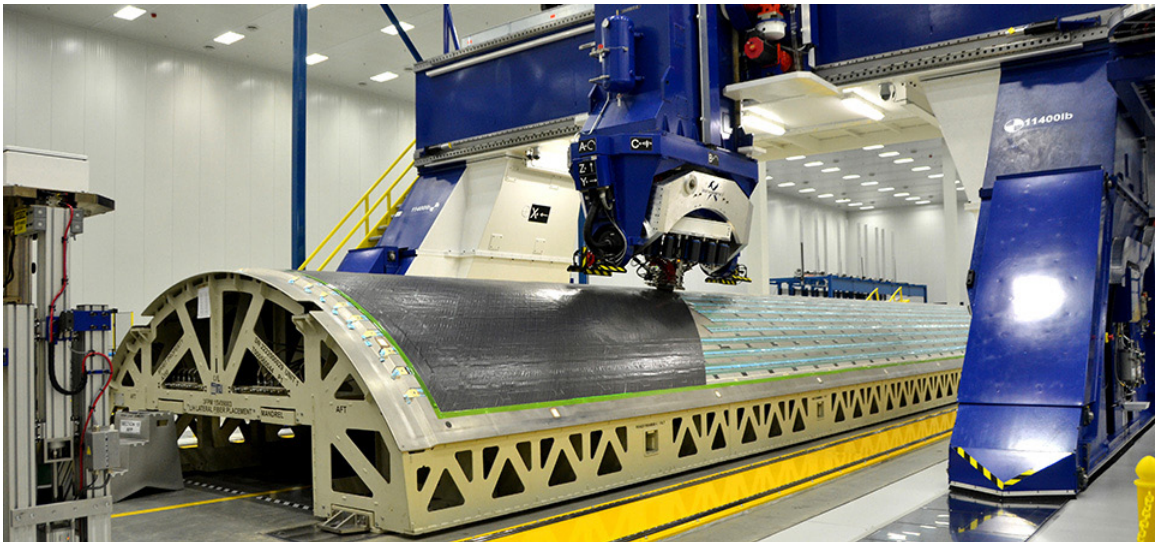
Figure 1.1: Production of a fuselage composite panel using automated fiber placement (AFP) technology (Courtesy of Electroimpact, Inc. See Appendix C.1 for copyright agreement).
